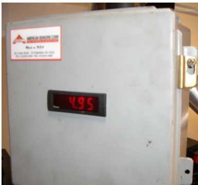
CB3000: Connection Box with LED display
