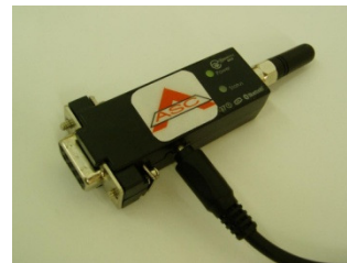
PDA-3000-PC: 1 Bluetooth transceiver (for sensor) + Bluetooth transceiver (for PC or Laptop)
